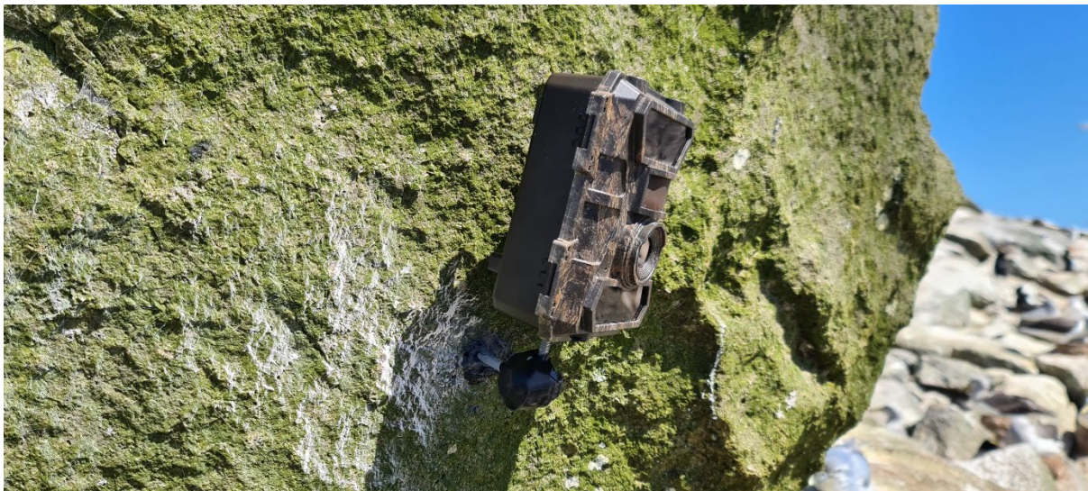
Figure 6. Time-lapse camera (Albatross 1) mounted to a overhang using eyebolts anchored in the rock.
