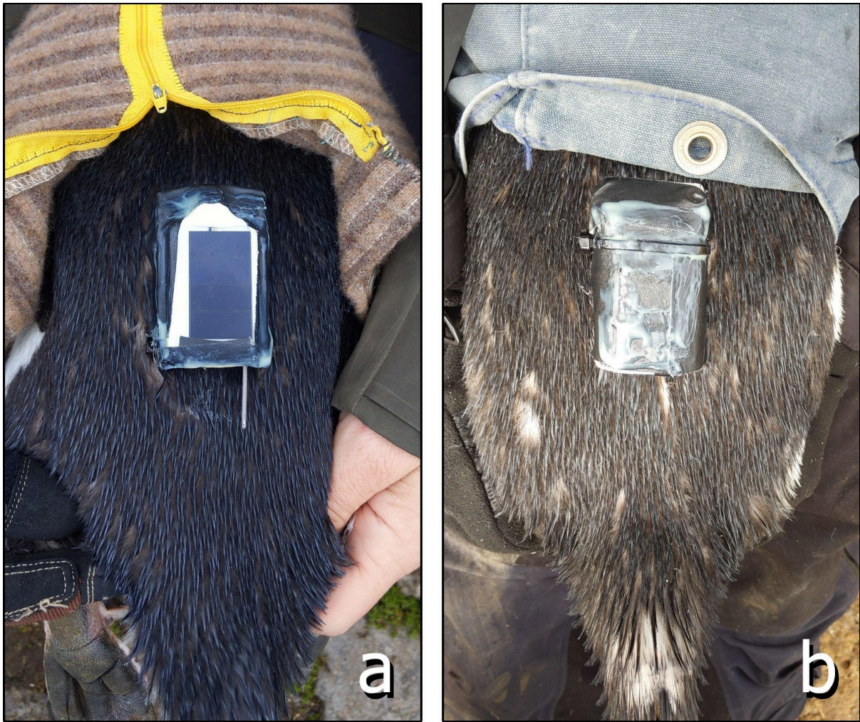
Figure 9. The two types of GPS dive loggers used during the incubation period on Erect-crested penguins. (a) AxyTrek Remote with solar panel, (b) standard AxyTrek Marine (both devices manufactured by TechnoSmart, Italy).
