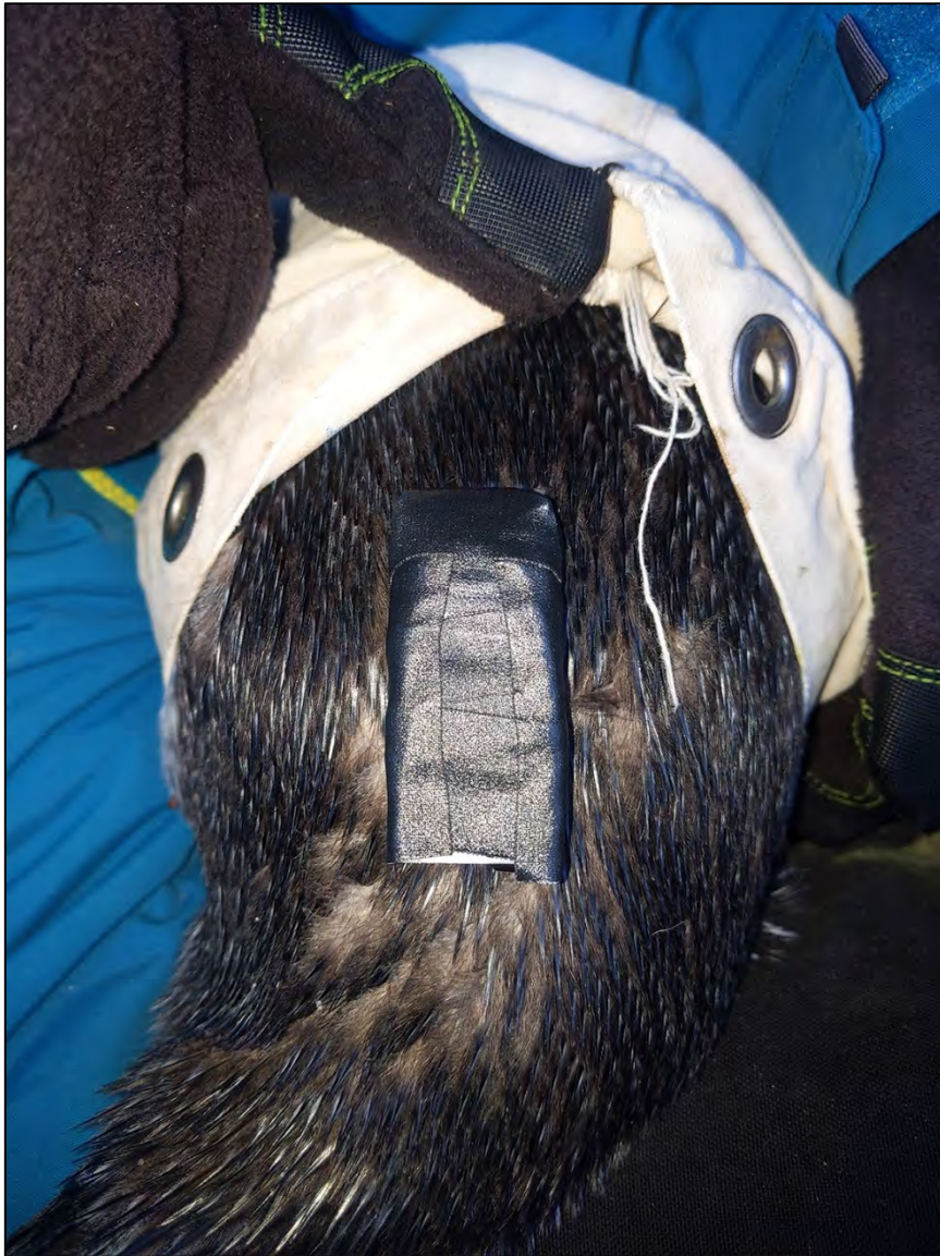
Figure 8. Axy-Trek Marine with 800 mAh battery attached to the lower back of an Eastern Rockhopper penguin. The device weighs about 20 g.
