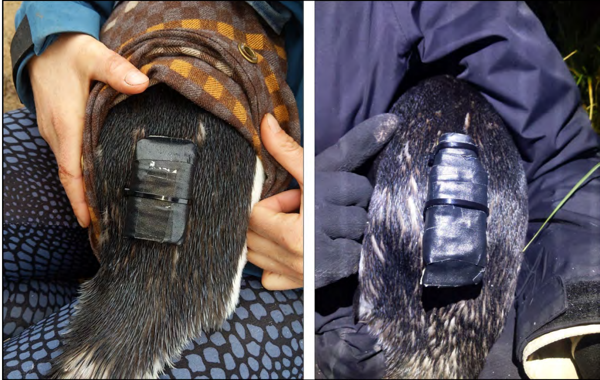
Figure 5. GPS dive logger (left) and PenguCam combined with TDR (right) deployed on Erect-crested penguins. The GPS logger (Axy-Trek with 2000 mAh battery) weighs 50 g. PenguCam and TDR weigh in combination ca. 95 g.
