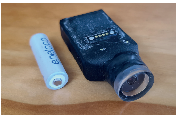
Animal-borne camera with an AA-battery for scale.
