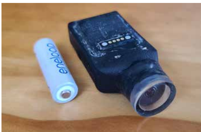
Animal-borne camera with an AA-battery for scale.
